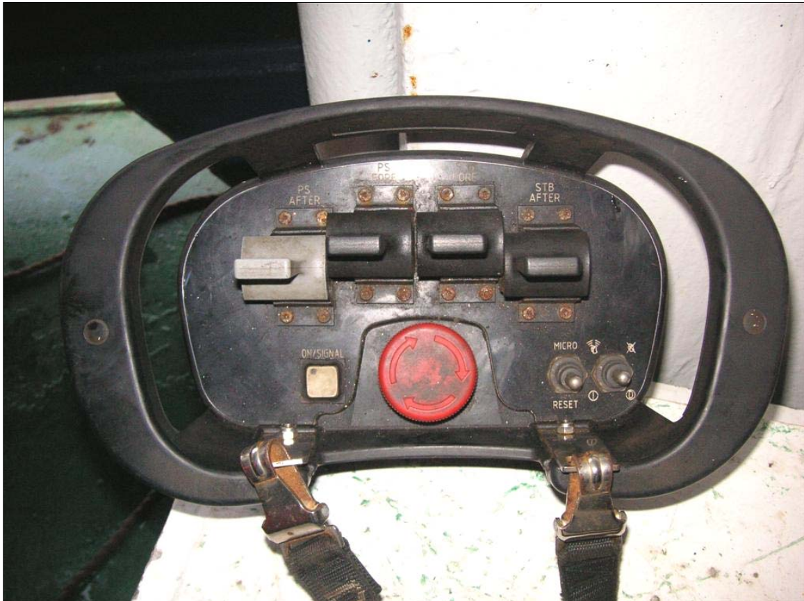
Photo: photo from 14 September 2005. Portable winch control (wireless)
