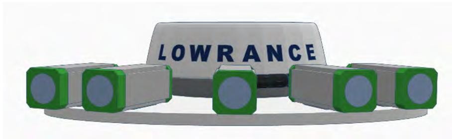
Figure 4.1: Sketch of the sensor platform. The five camera houses are looking forward in the ships heading. Camera units, CW-FM radar and GPS receiver plus IMU are fixed on the platform.
