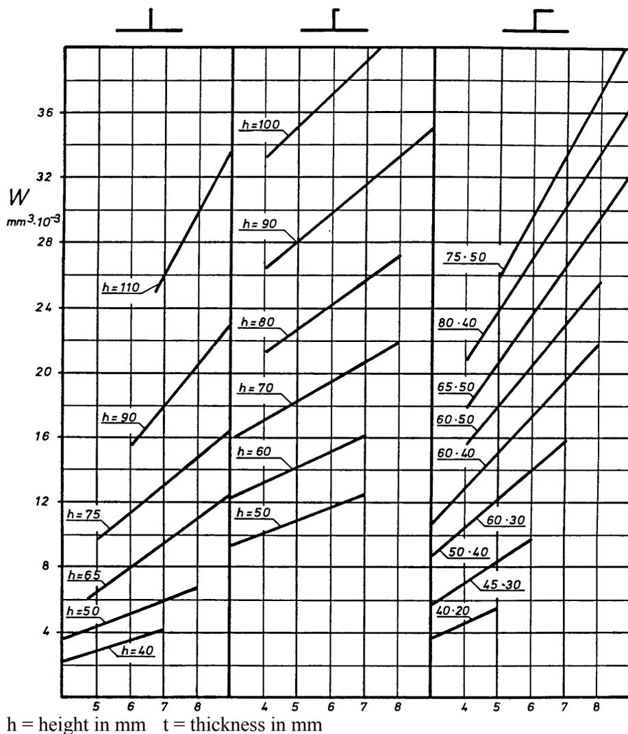
**Diagram showing section modulus for profiles, including plate section**
