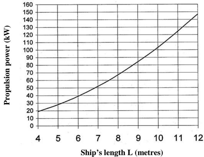
The diagram shows whether a vessel is covered by the order. The curve is made from the following formula:  $P \text{ (kW)} = L^2 \text{ (metres)} + 3$ .
